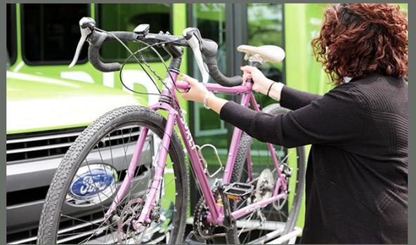
**4** If the rack is now empty, squeeze the handle and raise the rack to its stored position.
