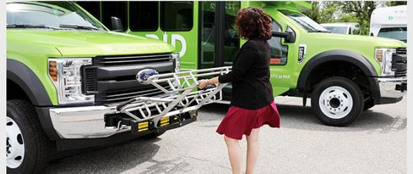
**3** Lift your bike and place both tires inside the wheel trays. The front tire should face the black rubberized support arm. **Always load bikes into the inner rack position (closer to the bus) first. The outer rack position should be reserved for a second bike.**
