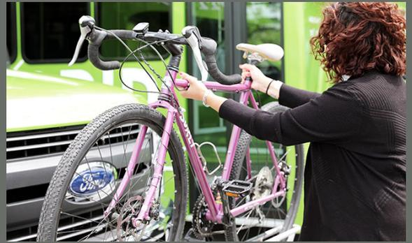
**4** Extend the black rubberized support arm, raise it over your front wheel, and then lower it (releasing the tension) to secure your bike. You can give your bike a quick shake to make sure that it's held tight.
